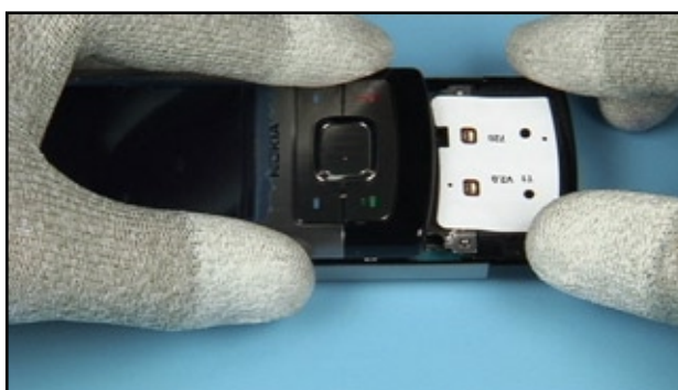
52. Push down the BOTTOM KEYMAT SUPPORT evenly.
